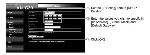
A confirmation screen appears. Press the [OK] button. The system restarts using the new IP address of VN-C20.lt takes about 1 minute for the camera to reboot.
